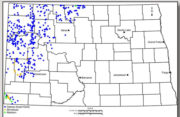
Figure 10. Active saltwater disposal wells in North Dakota, August 2015.
